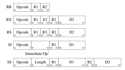
Because the "Immediate Op" text in the SI instruction is too long to fit in its box, DFORMAT places the text below the box and connects it with a line (as it did twice in the PDP-8 instruction format in the abstract). This picture is described as follows:
